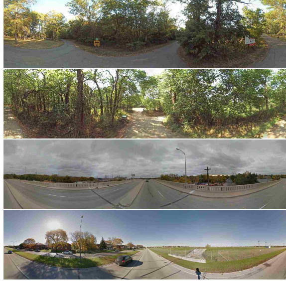
Figure 2.1: Example panoramas that our system uses to estimate the safety star rating. The top two are rated 1 star, the most dangerous. The bottom two are rated 5 star, the safest.
